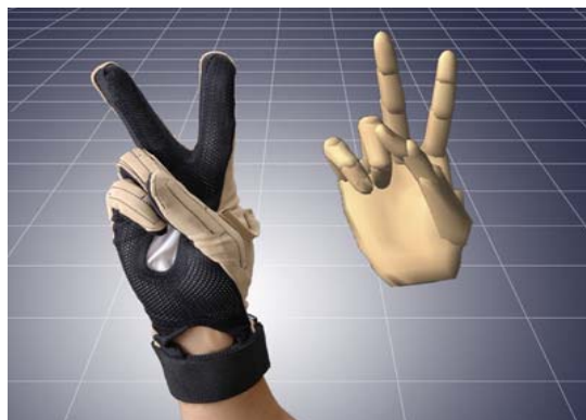
Hand feature extraction (Cyber-glove)
